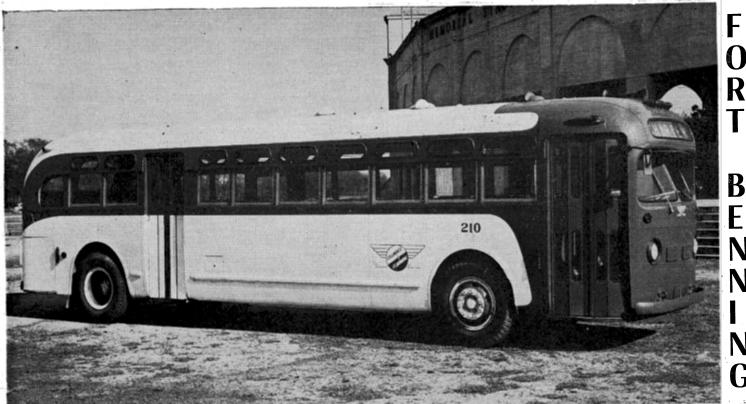
One of the new 40-passenger Diesel Hydraulic drive buses which operate on 20 minute schedule between Columbus and Fort Benning.
