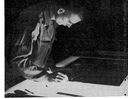
PFC. VINCENT GERMANN, JR., LEFT, SENSITIZES A ZINC PLATE WHILE SGT. BOBBY PRESTON, RIGHT, READIES A NEGATIVE USED TO TRANSFER SENSITIZED PLATE
